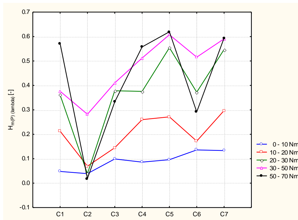
Fig. 2. The indicator values of information capacity H_m for \lambda and transient with n = 1100 rev / min and load change from T_{iq} = 0 Nm to T_{iq} = 70 : P - delayed injection timing, C1 - C7 - combinations of explanatory variables
