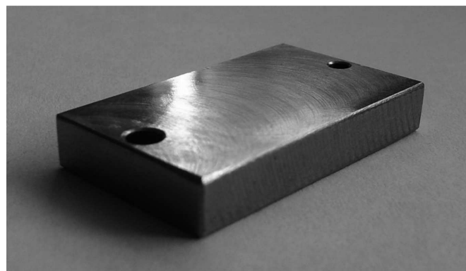
Fig. 3. A sample of the Ti6Al4V alloy used for tribocorrosion test
