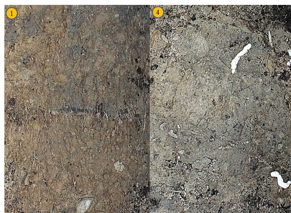
Fig. 16. Root penetration at the unvegetated slope surface. Depending on the subsoil the roots cling into the surface (clay layer, left) or almost not (ash/silt mixture, right). Flume 2, test sections 1 and 4, original unvegetated conditions
