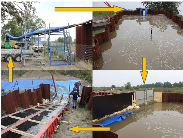
Fig. 6. Water cycle for the overflowing tests: pump, reservoir, shutters and flumes
