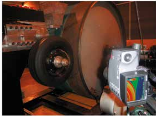
Fig. 3. Roadwheel facility with outer drum of 2.0 m diameter
