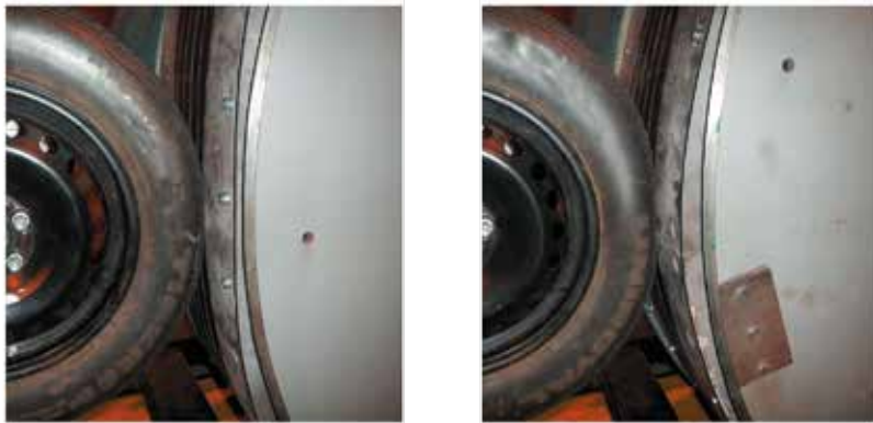
Fig. 4. Minimum (left) and maximum (right) dynamic deflection of the tyre rolling on the sinusoidal replica road surface
