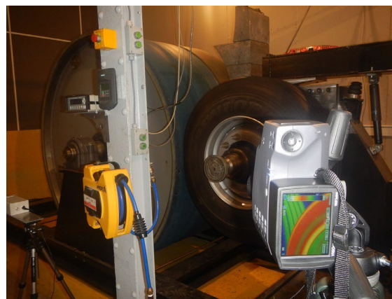
Figure 2. Roadwheel facility at TUG with external drum of 2.0 m diameter.
