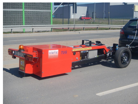
Figure 3. Trailer R 2 Mk.2 used to measure rolling resistance of passenger car tyres on Stone Mastic Asphalt SMA8.
