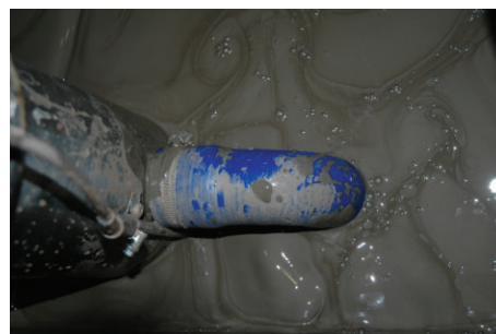
FIGURE 7: The picture of drilling mud containing gas, drilling mud from Sowia Góra borehole.
