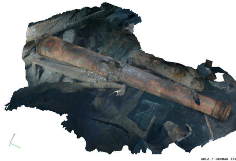
Fig. 16 A fragment of a point cloud generated from underwater photographs [10].
