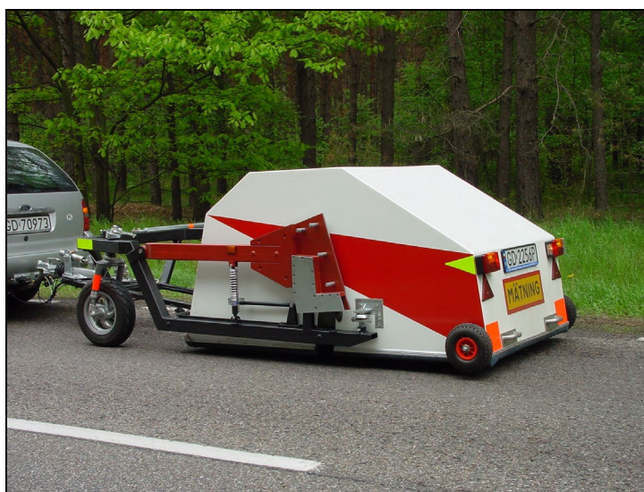
Figure 7. Trailer Tiresonic Mk.4 designed and built by TUG for CPX measurements.
