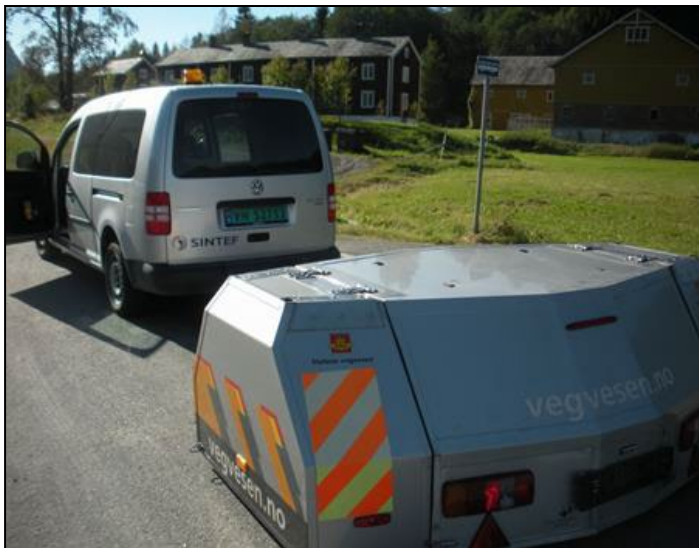
Figure 9. CPX test trailer used by SINTEF, Norway
