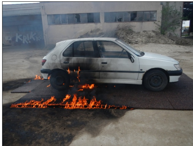
Figure 13. Car fire 260 s after ignition.
