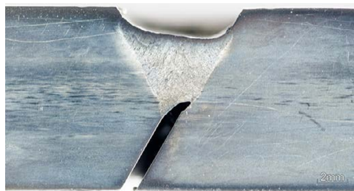
Fig. 6. Cross-section of the joint welded in air: specimen P1, q_{el} = 0.87 kJ/mm; the lack of welding imperfections; etchant: Beraha
