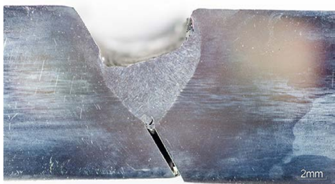
Fig. 3. Cross-section of the joint welded under water: specimen W2, non-saline water, q_{el} = 1.11 kJ/mm; the lack of welding imperfections; etchant: Beraha
