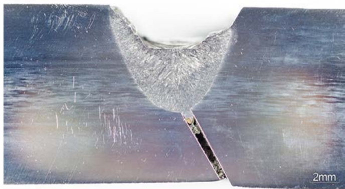
Fig. 2. Cross-section of the joint welded under water: specimen W1, non-saline water, q_{el} = 1.11 kJ/mm; the lack of welding imperfections; etchant: Beraha
