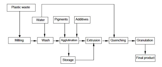
**Figure 2.** Stages of mechanical recycling (Aznar et al. 2006).
