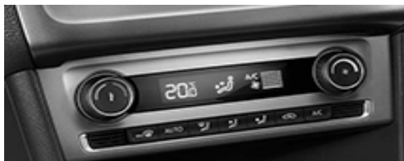
Fig. 3. Climatronic control panel [6]
