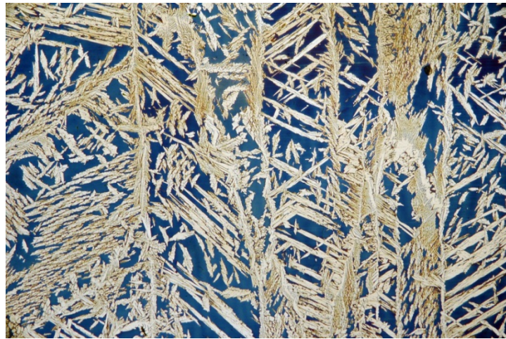
Fig. 7. Weld metal microstructure (W1). Magn. 100x
