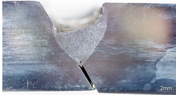
Fig. 3. Tekken sample W2. Welding bead performed underwater with heat input 1.1 kJ/mm. No imperfections. Beracha's etch.
