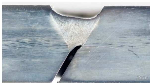
Fig. 6. Tekken sample P1. Welding bead performed on the air with heat input 0.87 kJ/mm. No imperfections. Beracha's etch.
