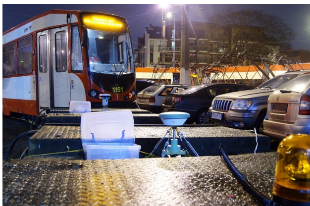
Figure 2: Measuring set with Leica Viva GS-15 and GS-12 receivers mounted on a tram bogie (photo by Jacek Szmaglinski).
