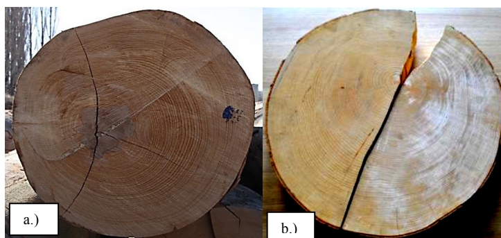
Fig. 1 a.) Eccentric pith, b.) Shiny appearance of tension wood
