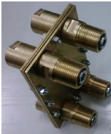
Figure 1. View of PHE prototype with minichannels.
