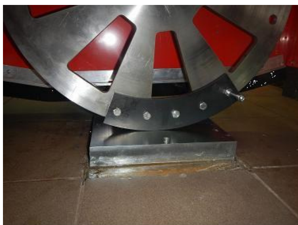
Figure 15. Calibration of R2 Mk.2 trailer - rutting influence.
