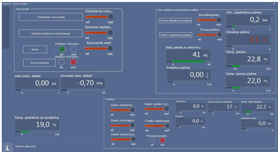
Fig. 5. Sample turbine engine station operation parameters monitored by the operator [3]
