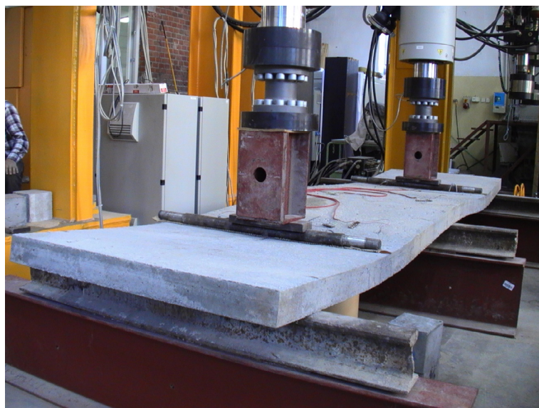
Fig. 7. Slab B-2 shortly before its failure
