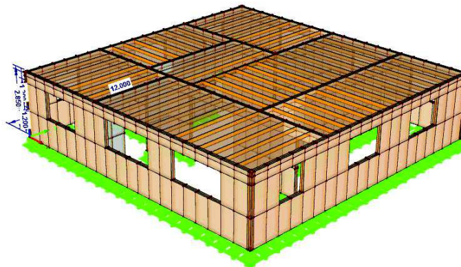
Figure 11. Numerical model of the whole wood-frame house
