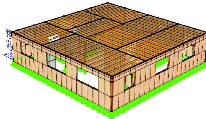
Figure 11. Numerical model of the whole wood-frame house
