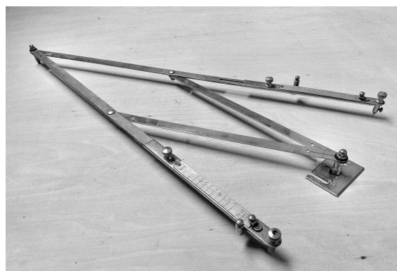
Illustration 2: Collection of Prof. H. Limon: Nickel-plated pantograph, company Cav. Pierro, Brevetto Fumagalli – photo K. Krzempek
