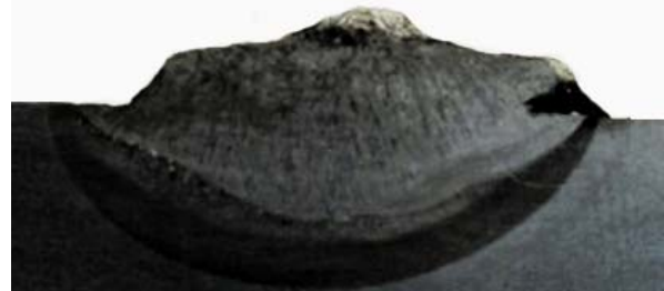
Fig. 3. Cross sections of weld beads: a) sample 5 - pitch 55%, b) sample 6 - pitch 89%, c) sample 7 - pitch 100%
