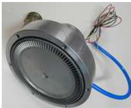
Figure 6: Nozzle disc of microturbine 1st stage.
