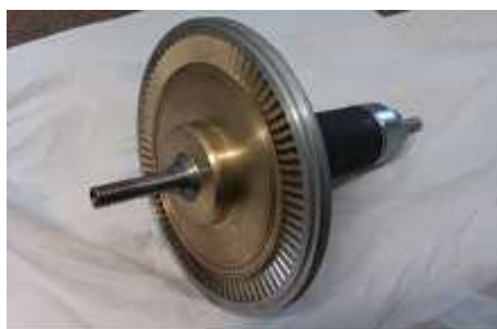
Figure 4: Turbine rotor disk with generator rotor.
