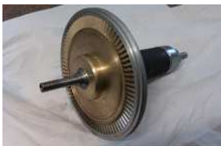
Figure 4: Turbine rotor disk with generator rotor.
