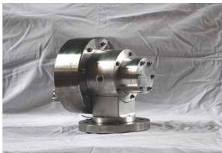
Figure 3: View of vapour ORC microturbine.
