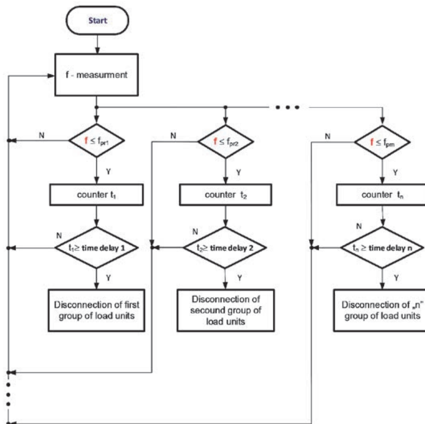
Fig. 5. Underfrequency load shedding automatics algorithm implemented in load model
