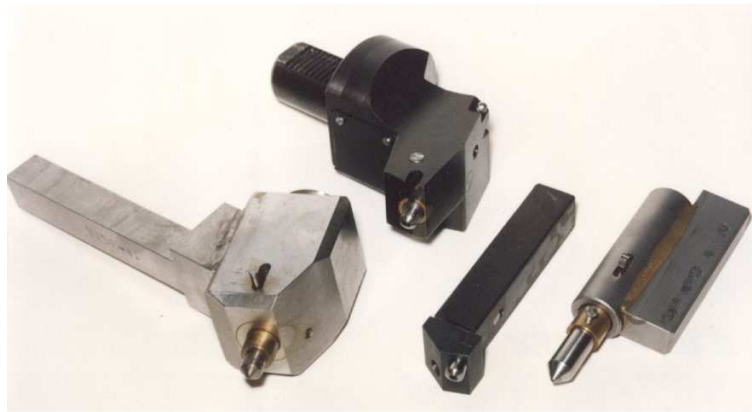
Fig. 2. Sliding burnishing tools for lathes were designed and made by Gdansk University of Technology
