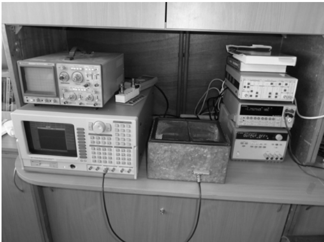
Fig. 5. A photography of laboratory setup for testing exhaled air samples using DC resistances and their fluctuations
