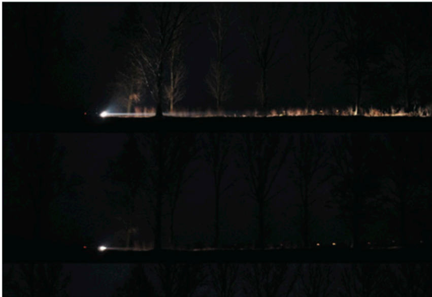
Fig. 5. Comparison between the ranges of road illumination. From the top: sports headlamps, main-beam headlamps, dipped-beam headlamps (by: Krzysztof Stryjek)
