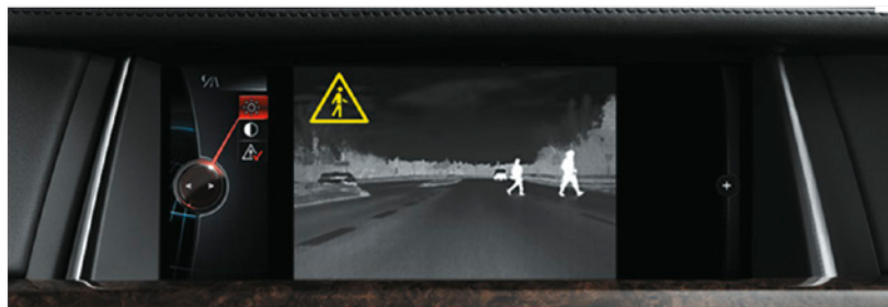
Fig. 11. View of recognized pedestrians displayed by the BMW Night Vision system (source: BMW Poland)
