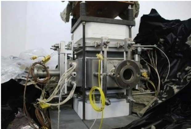
Fig. 39 – 1 kW MCFC stack, Warsaw University of Technology.
