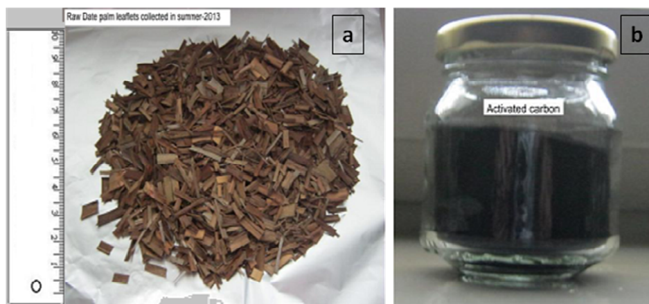
Fig. 2. Rawpalm leaflets (a), and activated carbon from DL storage into colsed glass container (b)
