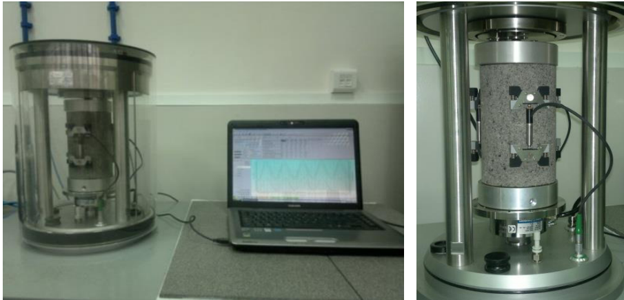
Fig. 2. The specimen inside the simple performance tester.
