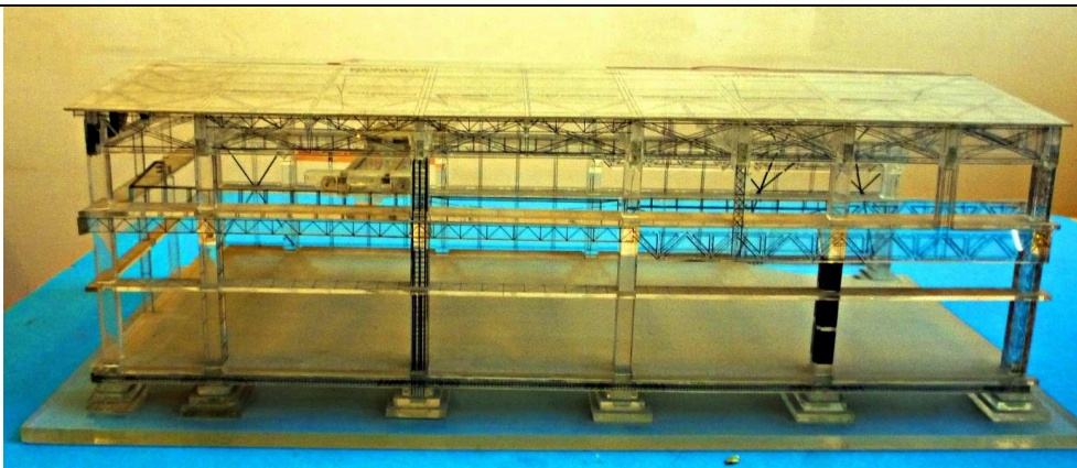
Figure 6: The model of an industrial hall with a crane. The options of columns of different structures are shown
