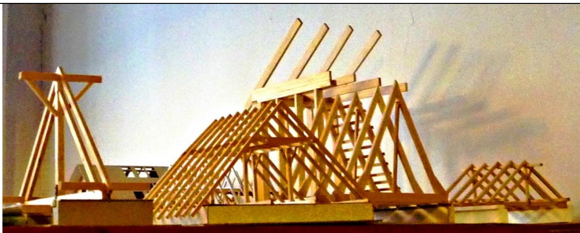
Figure 11: Models of wooden roof trusses made by students of the Faculty of Architecture
