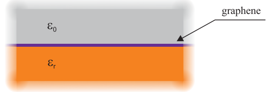
Fig. 8. Graphene transmission line, where \epsilon_r = 11.9 .
