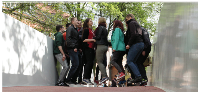
Fig. 12. Example tests: static loading with concrete road slabs (top); dynamic, synchronous jumps by a group of pedestrians (bottom)
