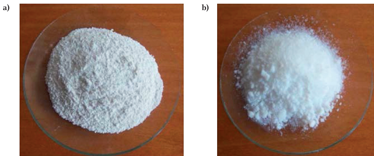
Fig. 1. Comparison of silica fillers characterized by different particle size: a) submicron-sized silica ( 0,2 \mu\text{m} ), b) nano-sized silica ( 12 \text{ nm} )
