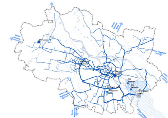
Figure 9 Water supply: existing network
