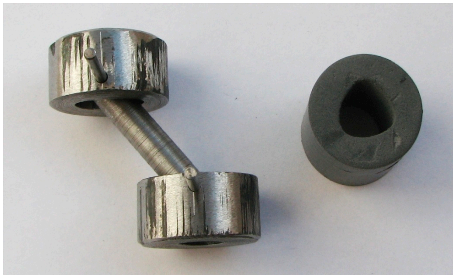
Figure 5. Components of the prototype PB: pin-ended steel core with the anchor plates ( left ), and a polymer cylinder with a centrally located hole ( right ).
