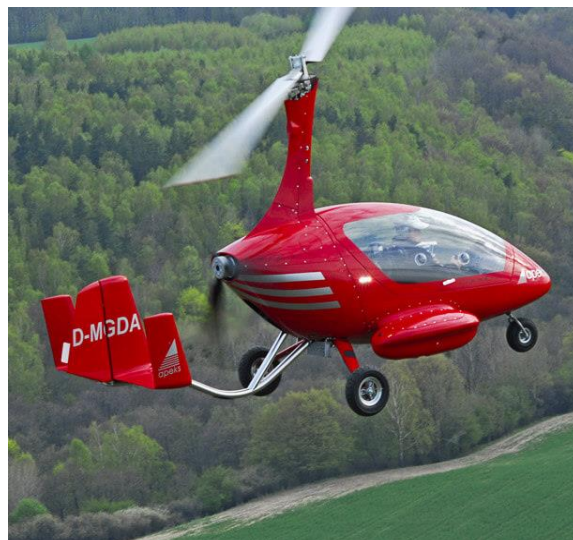
Fig. 4 Gyroplane, which is used for mapping using Airborne Laser Scanning
