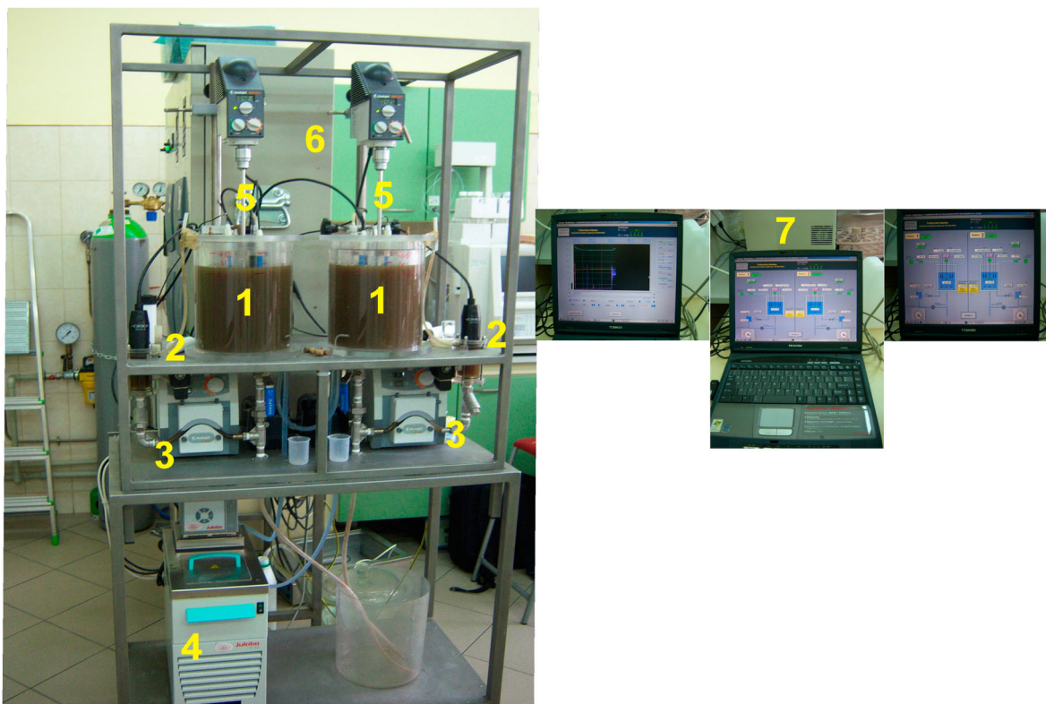
Photo 1. Experimental setup. 1 – batch reactors; 2 – units for the continuous measurement of oxygen uptake rate (OUR); 3 – peristaltic pumps; 4 – cooling/heating system; 5 – mechanical stirrers; 6 – control box; and 7 – computer control and data acquisition system.
