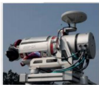
Fig. 2. Riegl VMZ-400 Horizontal mounting [5].
