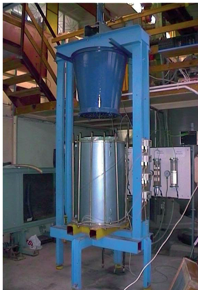
Fig. 3 Calibration chamber at GUT [24]
