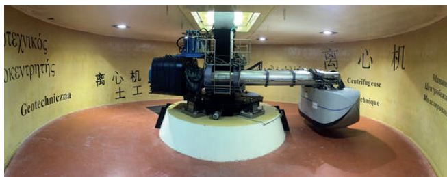
Fig. 1. Geotechnical centrifuge at Ifsttar [19].
