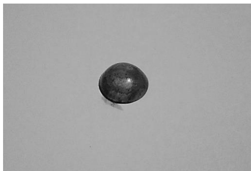
Fig. 1. The contact lens with the obtained coating /immersion for five minutes/
