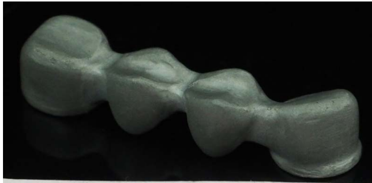
Fig. 3. The prosthetic bridge obtained by selective laser melting method (SLM) after sandblasting
