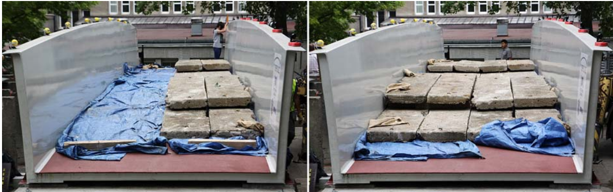
Figure 5. Footbridge loaded with ballast during static tests
