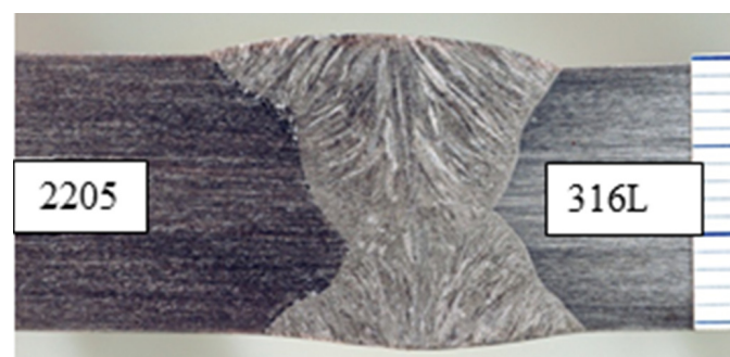
Fig. 2. Macrostructure of dissimilar 2205 – 316L welded joint
