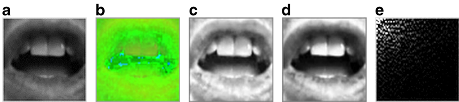
Fig. 26 Visualization of ROI frame analysis for the following images a ) original, b ) in HSV, c ) after equalization, d ) after filtering with CLAHE algorithm, e ) DCT parameters
