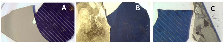
Fig. 3. Pictures of samples A-before the etching process, B-after 1 h of etching with 1 M HNO 3 50 °C, C-after 15 min of etching with 1 M NaOH 30 °C with stirring speed 250 rpm.
