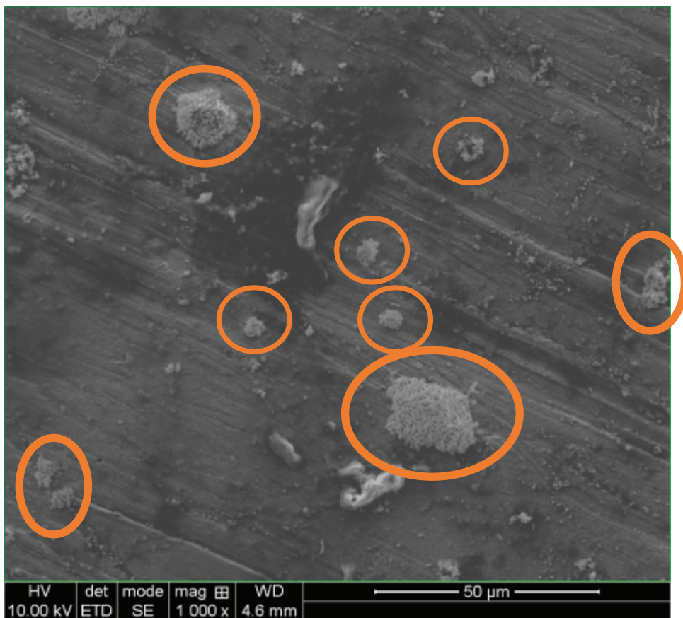
Fig. 6. Biofilm on the surface of the implant
