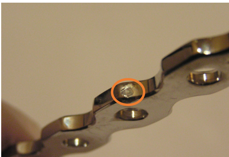
Fig. 4. Plates used for joint bones with corrosive focus
