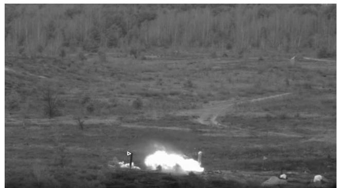
Fig. 14 Jet fire associated with shooting hydrogen cylinder.
