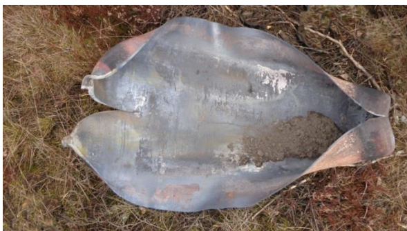
Fig. 5 Fully ruptured acetylene cylinder
