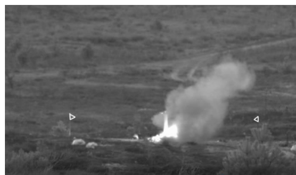
Fig. 7 Jet-fire after puncturing acetylene cylinder
