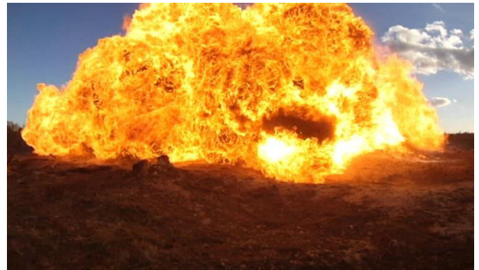
Fig. 21 Fireball developed after shooting through LPG cylinder
