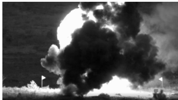
Fig. 6 Fireball during acetylene cylinder explosion (distance between triangle markers is 10 m)
