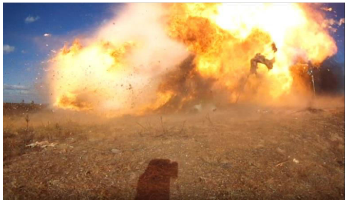
Fig. 20 Hydraulic blow of the LPG cylinder with combustion
