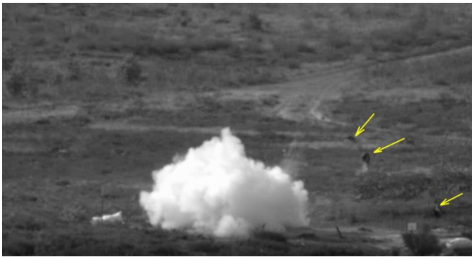
Fig. 18 Hydraulic blow of the LPG cylinder without combustion; arrows indicate shrapnel
