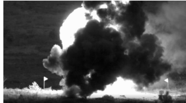
Fig. 6 Fireball during acetylene cylinder explosion (distance between triangle markers is 10 m)
