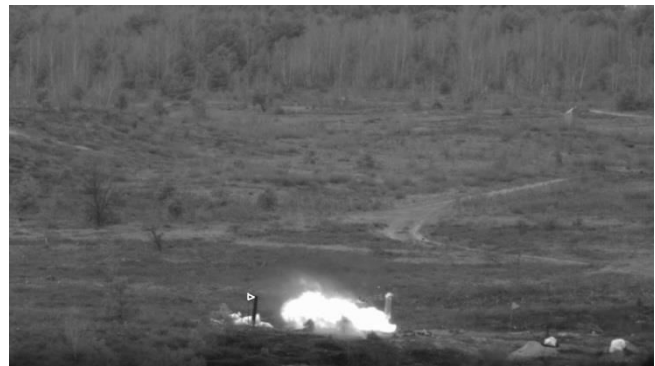
Fig. 14 Jet fire associated with shooting hydrogen cylinder.
