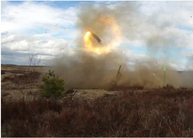
Fig. 11 Oxygen cylinder rotating after hit by bullet
