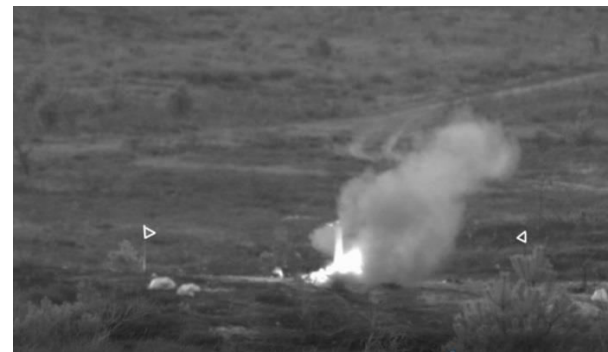
Fig. 7 Jet-fire after puncturing acetylene cylinder
