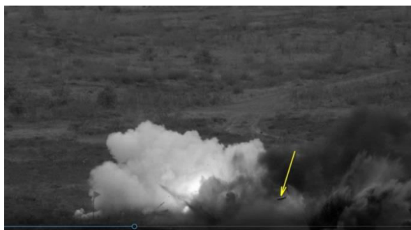
Fig. 15 Explosion of methane cylinder; the arrow indicates big shrapnel that moved over 500 m.
