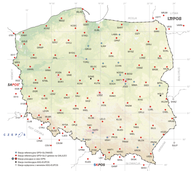
Figure 2: Distribution of the ASG-EUPOS system stations in Poland ( www.asgeupos.pl , state on the 21 February 2017)
