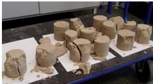
FIGURE 9. Samples after UCS test
