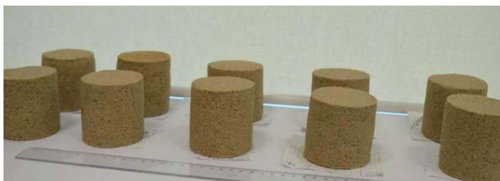
FIGURE 4. Solid sand with xanthan gum samples
